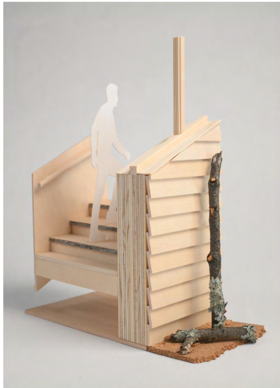
Detail model showcasing interior vs. exterior connection
